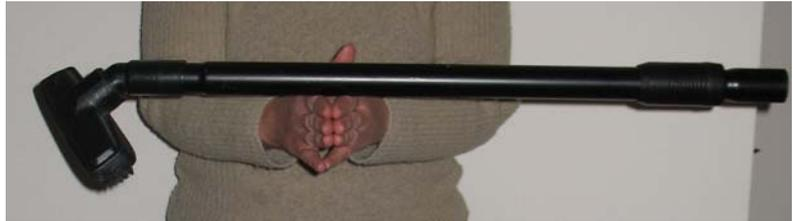
located. If you are using a metre stick and want the centre of mass to be somewhere other than the 50-cm mark, just attach one or more clamps to the stick. Balancing the object on the fingers allows the students to find the location of the centre of mass. On the photo above, the vacuum cleaner brush and holder are balanced on the top of my forefingers. This is where the centre of mass of the brush-holder system is located.
